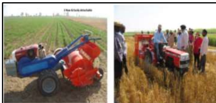
Figure 9.6: Low Powered Tractor Drawn Turbo Happy Seeder
