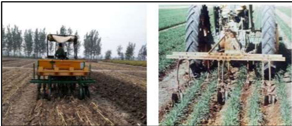
Figure 9.8: Inclined plate planter with double disc furrow openers sowing wheat on PRBs (left) and earthing up/weeding in PRBs in wheat (right).
