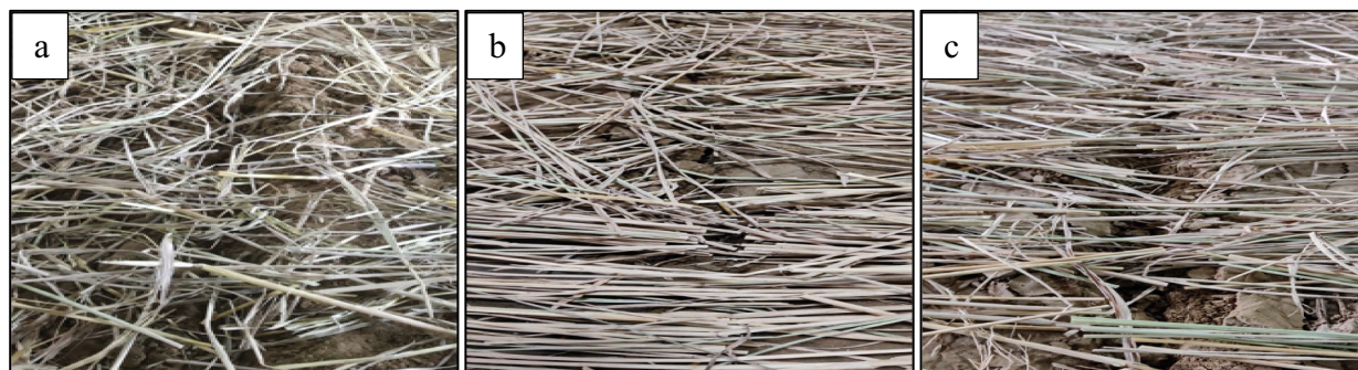
Fig. 8. Straw cutting and furrow grooves opening mechanism of (a) SD, (b) ITRC and (c) DD furrow openers.
