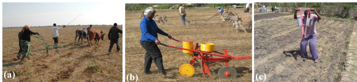
Fig. 3. Examples of smallholder tillage implements in SSA (a) ripper for direct seeding in Zambia (b) animal-drawn direct seeder and fertilizer distributor in Tanzania, and (c) mechanical jab planters for manual direct seeding and fertilizer application.
