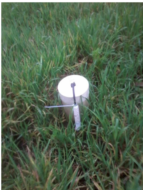
Figure 4.1 Soda Lime trap in field, showing main chamber with CO 2 scrubber on breather hole
